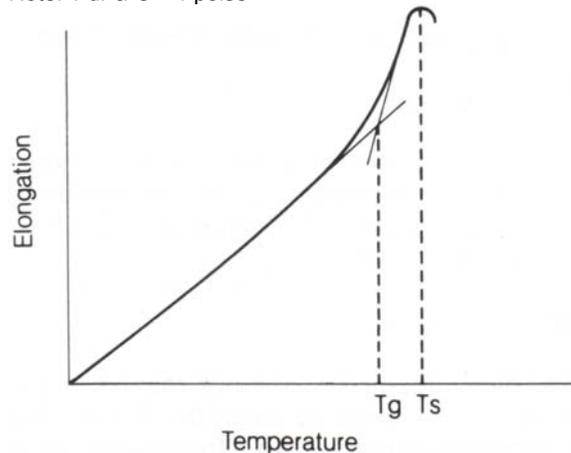
Fig. 2 Thermal Expansion Curve.
