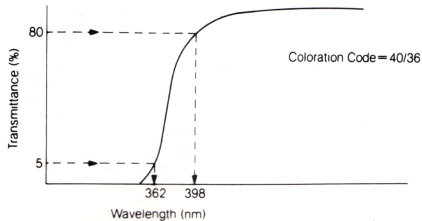
Fig. 1 Designation of the Coloration Code in Spectral Transmittance curve.
